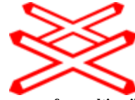
Warning cross for multi-rail railway crossing
