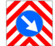
Mandatory passage for works vehicles
