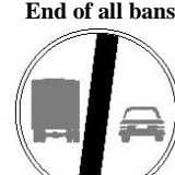
End of overtaking ban for vehicles whose maximum gross weight exceeds 3.5 tonnes
